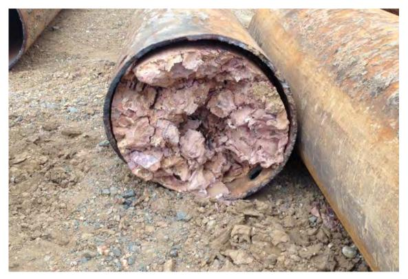
Photograph 4.1 Sinker pipeline blockage during the Western Basin Dredging and Disposal Project dredging works
