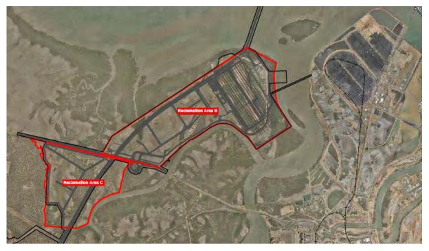
Figure 4.7 Wiggins Island Coal Terminal Project reclamation areas B and C
