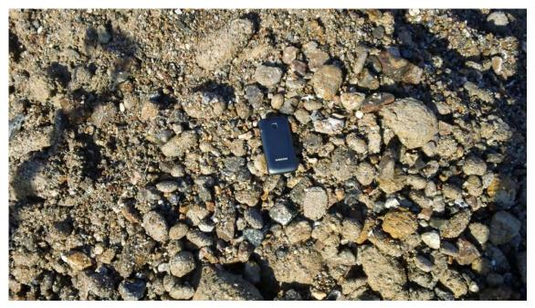
Photograph 3.1 Dredged material from the Western Basin Dredging and Disposal Project
