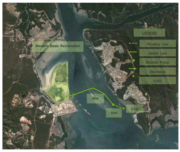
Figure 4.5 Western Basin Dredging and Disposal Project dredging and intertidal reclamation arrangement
