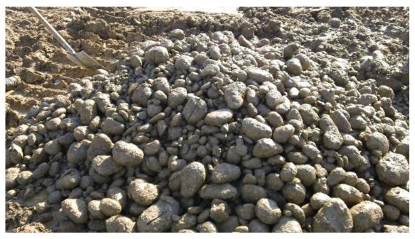
Photograph 3.2 Dredged material forming clay balls from the Western Basin Dredging and Disposal **Project**
